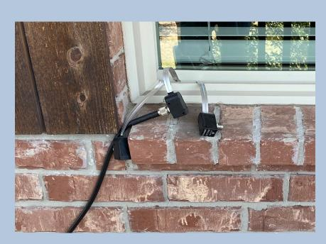
~.5 dB Insertion Loss @ 450 MHz
